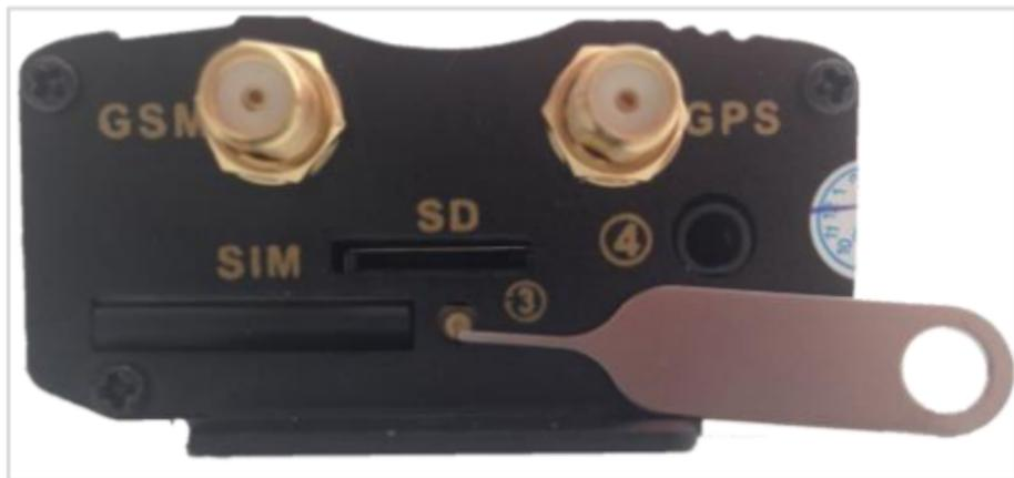
In order for the SIM card to be inserted into the tracker, the SIM card compartment must first be opened and the so-called SIM **card slot** removed. To do this, press the yellow small button on the front of the device using a pointed object (see figure with needle). Insert the SIM card into the card slot. The **gold contacts must point upwards**. As a next step, the SIM **card slot with SIM card** can be inserted again into the finder.
