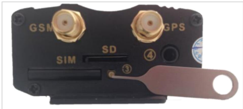
The SIM card used must be in the **standard format**. In order for the SIM card to be inserted into the tracker, the SIM card compartment must first be opened and the so-called **SIM card slot** removed. To do this, press the yellow small button on the front of the unit using a pointed object. The top picture shows the opening using a SIM card needle. *This is not included in the standard delivery scope.*
